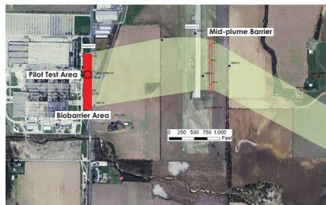
Extent of TCE plume (green) and location of pilot test area and full scale biobarrier indicated in red (from Kovacich et al., 2007)
